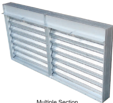
Multiple Section (2 units of single section connected together), Out of Airstream, automatically fully close when temperature reaches 165°F (74°C) to prevent fire flow through
